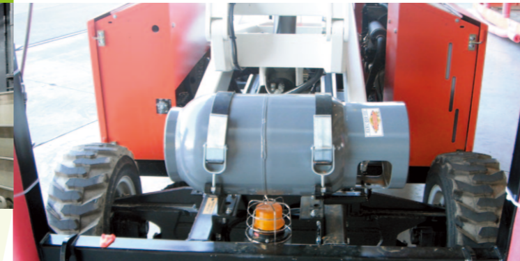
GSE with propane powered engine at HAECO Americas 港機（美洲）採用以丙烷作燃料的地勤支援設備
