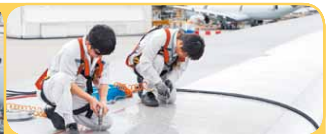
Technicians working on aircraft wing with fall arrest device
